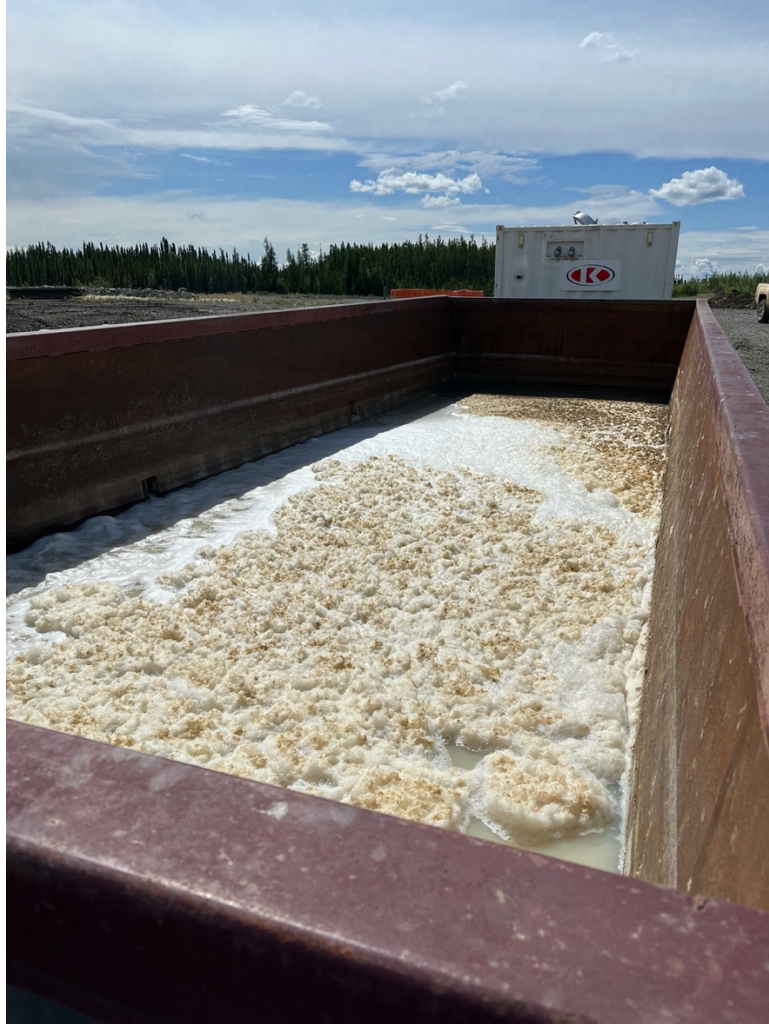
Figure 4.1: A large metal tank that is being used as a bioreactor, displaying the absence of any kind of barrier to prevent contamination from falling into the bioreactor.
