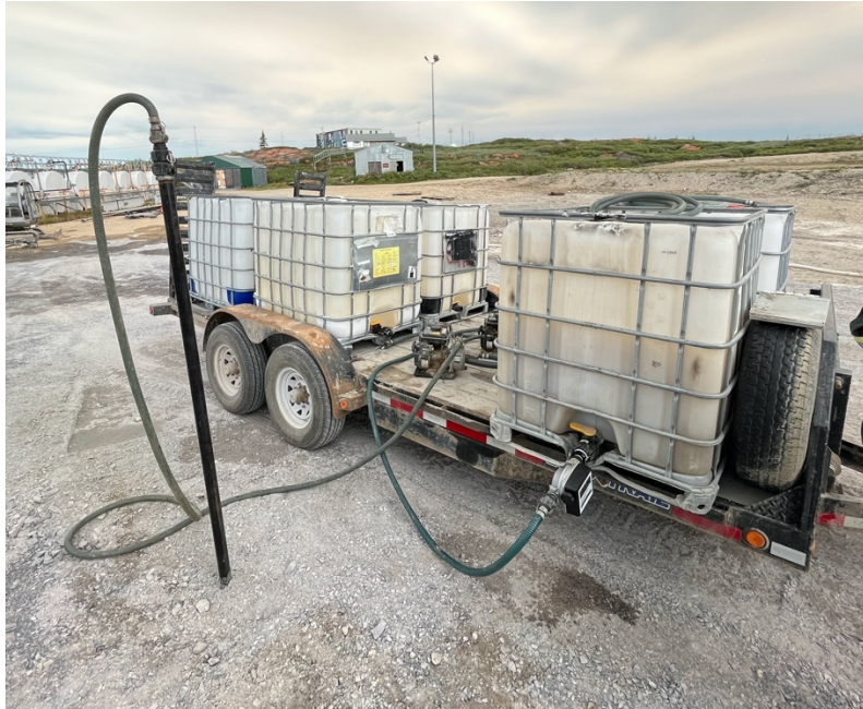
Figure 5.2: The 1000 liter tanks used for transporting the bacterial amendment to each injection well in Churchill, Manitoba
