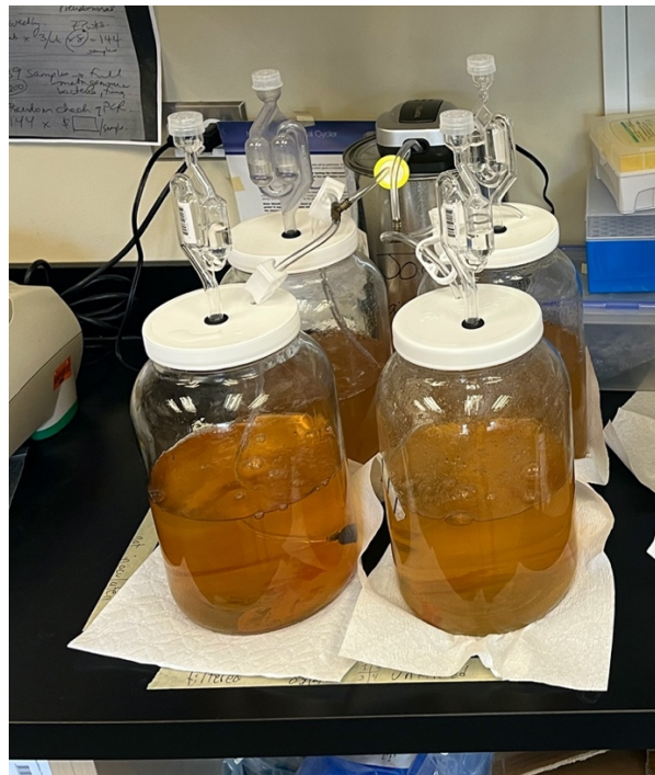
Figure 4.2: Bioreactor and airline set up to evaluate the effect of aeration on the bacterial community, noting the yellow syringe filter on only 1 of the air supply lines.
