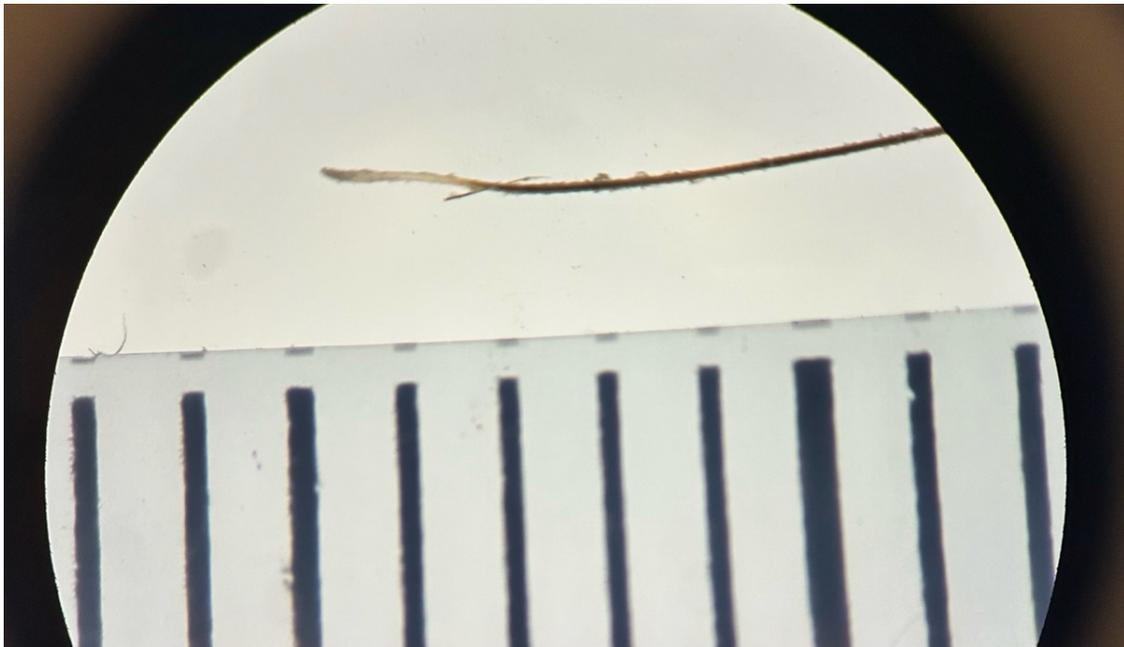
**Figure 4.** Image taken of a hair follicle underneath a dissecting microscope and used for measurement with ImageJ-2.
