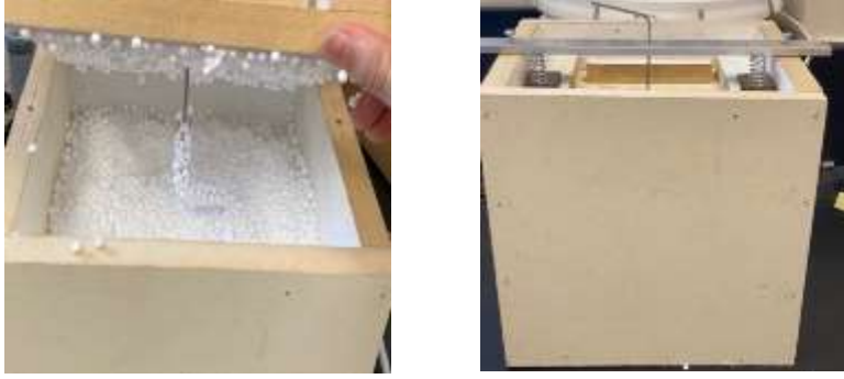
Figure 10. a) The polystyrene beads were placed inside of closed box. A thin rod was used to mix the polystyrene between trials. b) Springs were used on the lid to allow the beads to be compressed.
