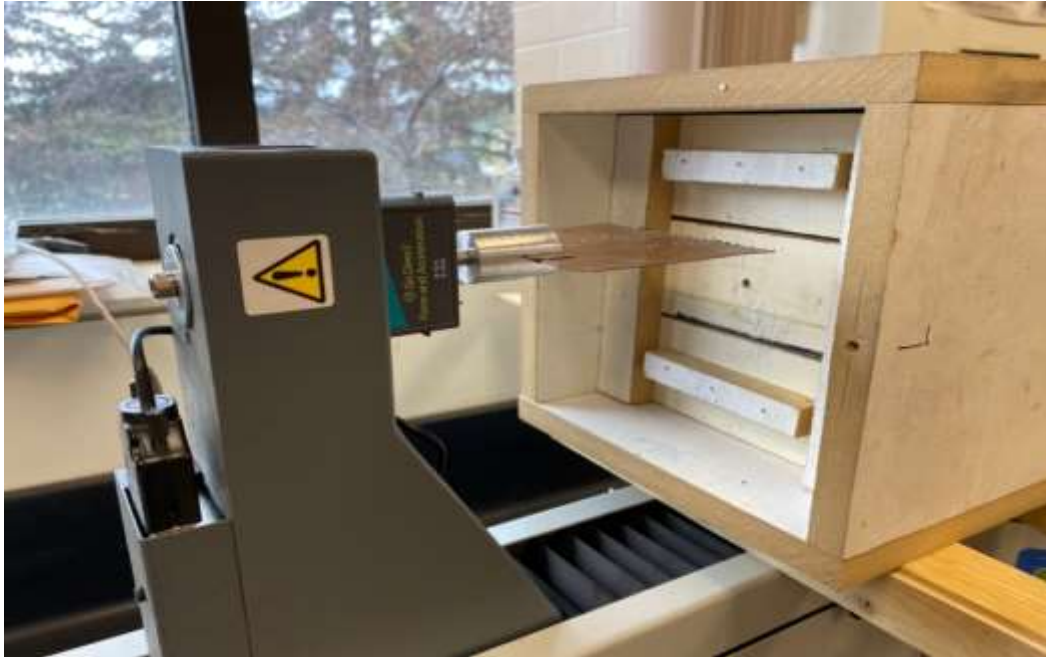
Figure 26. The box for the wet sand measurements marked with two levels in the cover, and the blade as it can be seen is matching level 2 before the insertion.
