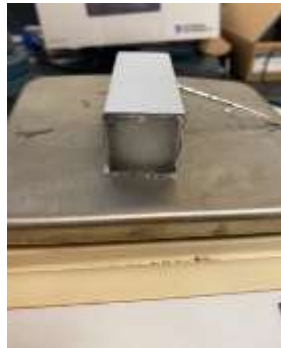
Figure 16 shows the square cylinder used to measure the density of the snow. Once the cylinder was filled, the mass was determined.
