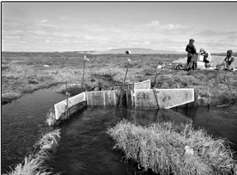
Figure 2-8 Upstream/downstream fish trap box 3 installed June 9, 2015 on the Pigeon Stream, Ekati (ERM, 2016). Data obtained from this trap were used for comparison to the cameras.
