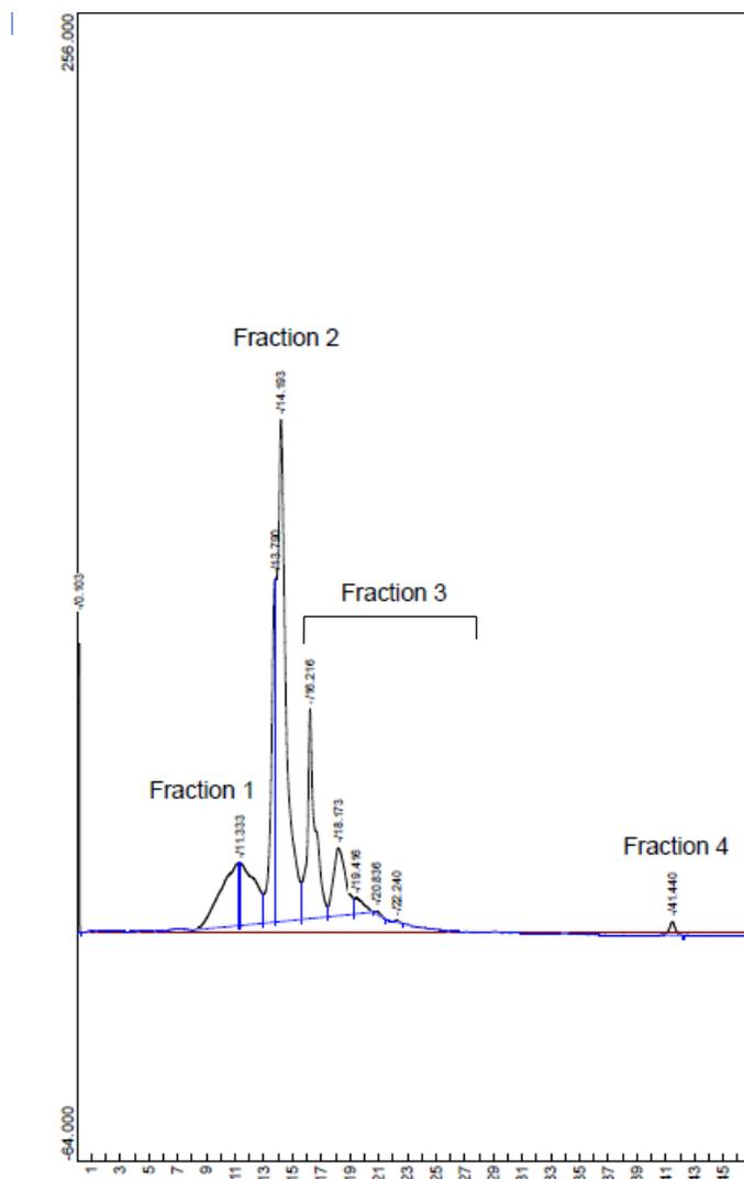
**Figure 9. Preparative reverse-phase HPLC of bioactive secondary metabolites in methanol.**
