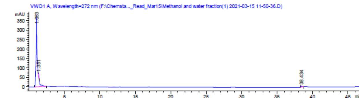
**Figure 8. Analytical reverse-phase HPLC chromatograms of bioactive secondary metabolites in methanol measured at 272 nm.**
