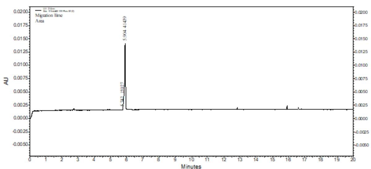
Figure 6. Electropherogram of 100 ppm indol45 run in 50 mM phosphate without the presence of micelles.
