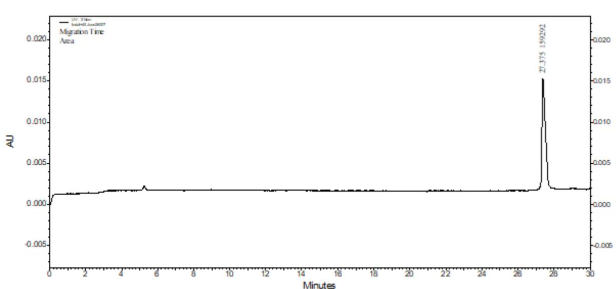
Figure 7. Electropherogram of 100 ppm indol45 run in 50 mM phosphate and 20 mM SDS with the presence of micelles.
