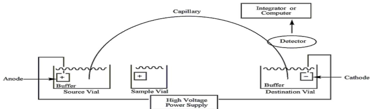
Figure 2. Schematic of the CE instrument set up.
