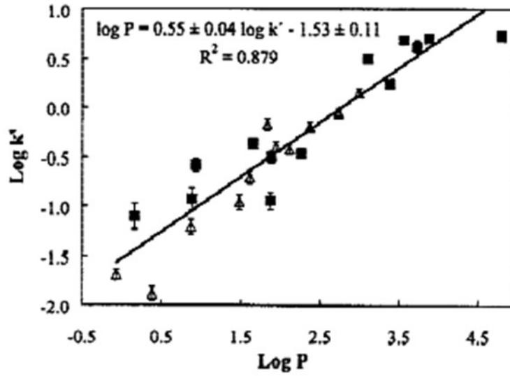
Figure 8. Calibration curve showing the relationship between calculated  $\text{Log } k'$  and known  $\text{Log } P$  values from which the  $\text{Log } P$  can be estimated from the equation of the line for indol/indol45 based on the calculated  $k'$  values.<sup>10</sup>
