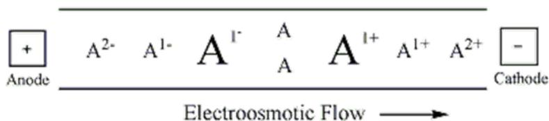
Figure 3. Schematic showing electrophoretic mobility of analytes.
