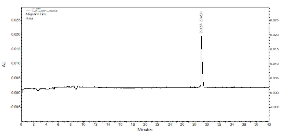
Figure 5. Electropherogram of 100 ppm indol run in 50 mM phosphate and 20 mM SDS with the presence of micelles.
