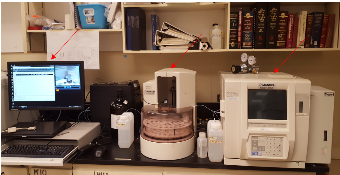
Figure 3. From left to right, arrows indicate the computer, the autosampler, and the analyzer.
