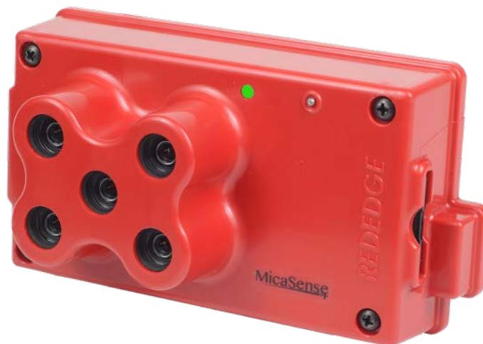
**Figure 16:** The MicaSense RedEdge® multispectral camera. This camera has 5 lenses, one for each spectral band, and 5, 1.2 mega-pixel sensor chips with a separate filter for each chip.
