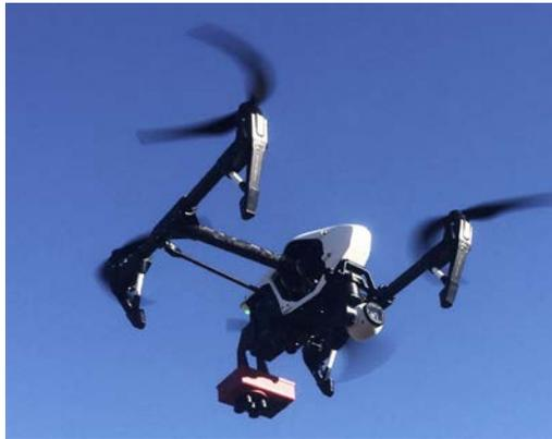
**Figure 3:** DJI Inspire 1 quadcopter with modified Zenmuse X3 and MicaSense RedEdge® simultaneously mounted.
