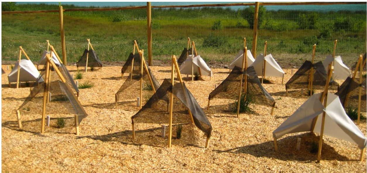
Figure 3.2: Shade structures covering individual rough fescue plants showing (front row, left to right): one layer of screen (44% shade), two layers of screen (66% shade), and full canopy shade treatments.
