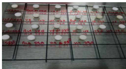
Figure 4: The discs used to test the antimicrobial activity of the cave bacteria with the disc diffusion assay. The sterile discs were dipped in bacteria fermentation broth and were left to dry on a glass plate in the fume hood.
