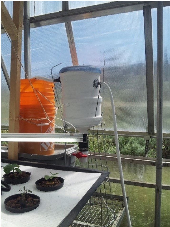
Figure 2. Biofiltration system: A raised 20L swirl filter(right) with inflow and out-flow water lines and a bottom valve for waste removal, and an open, three-tiered bucket filtration system (left). The the top bucket contained porous clay pellets, the second held gravel and the third had filter cloth and an outflow water line at the bottom.
