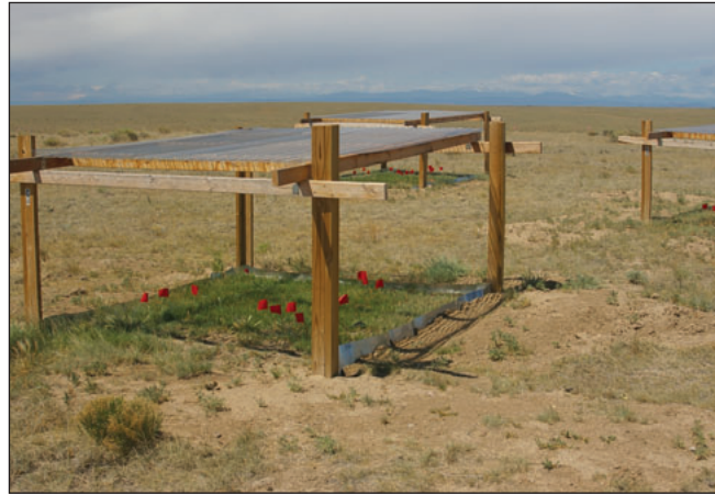
Figure 4. Example of the style of rain-out shelter proposed for the CDE to test the effects of drought in grasslands (from US, map location in Figure 3 is 12).
