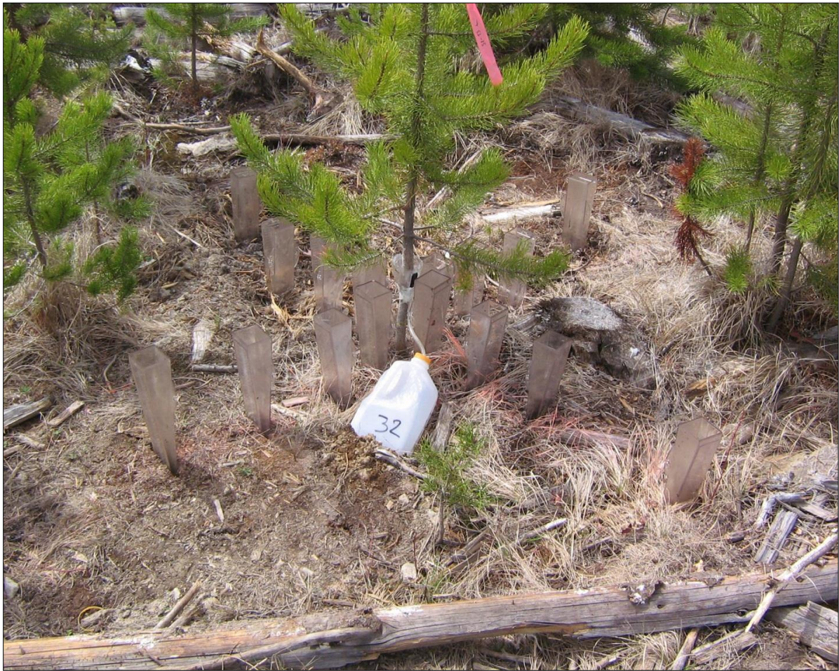
Figure 3.6: Stemflow and throughfall collection system for one of the selected study trees.
