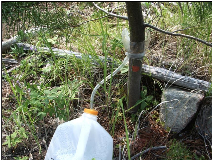
Figure 3.3. Stemflow collar and collection container used in Plots E and D.
