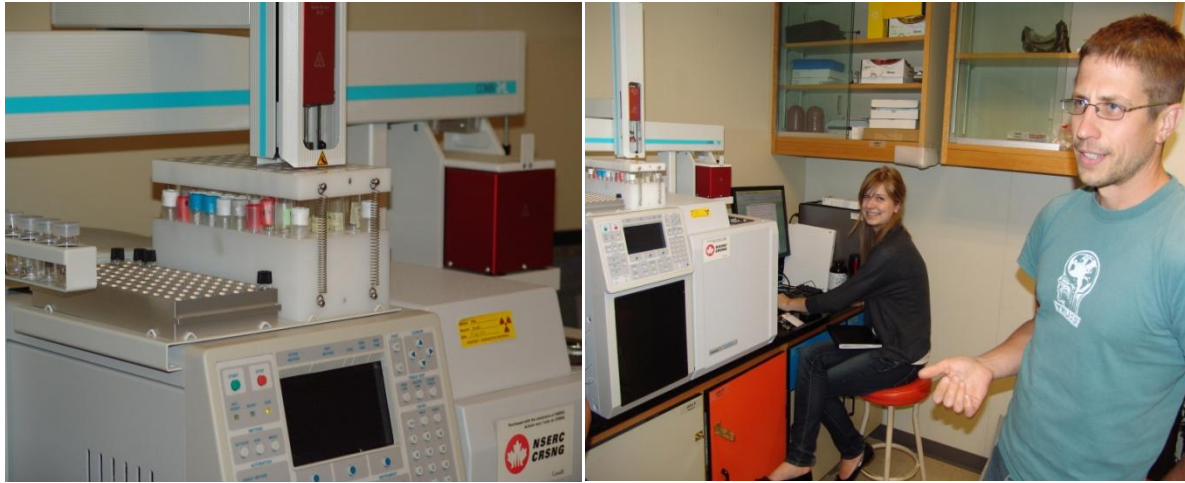
Figure 2.6. Measuring methane samples using gas chromatography.
