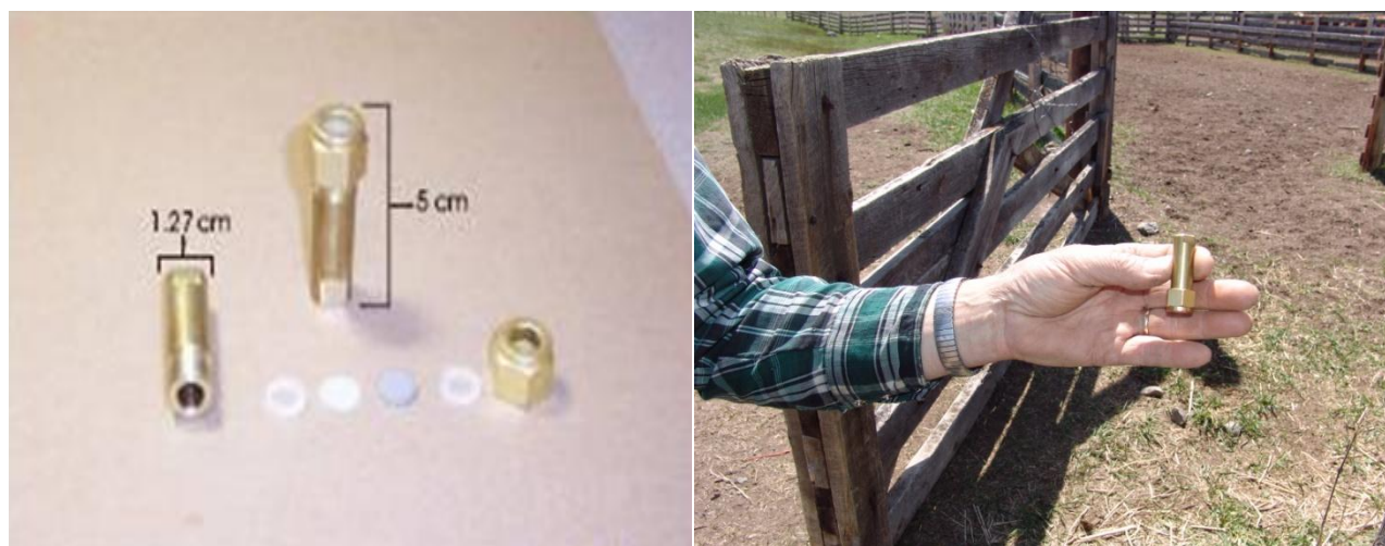
Figure 2.1. Permeation tube and components.
